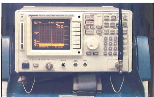
Figure 4—The Advantest R3361C spectrum analyzer used in the test.
